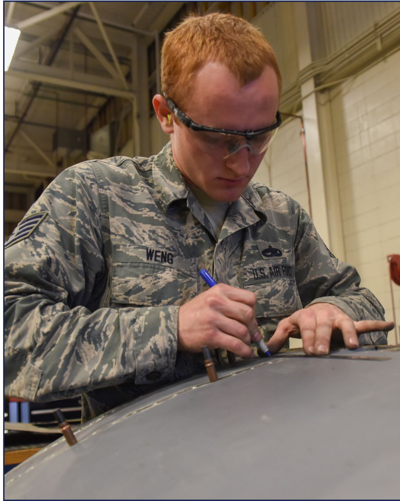
Staff Sgt. Robby Weng, aircraft structural repair mechanic, prepares a flush repair on a nose landing gear door. The repair was part of an extensive job replacing pieces of damaged skin of a C-130H.
