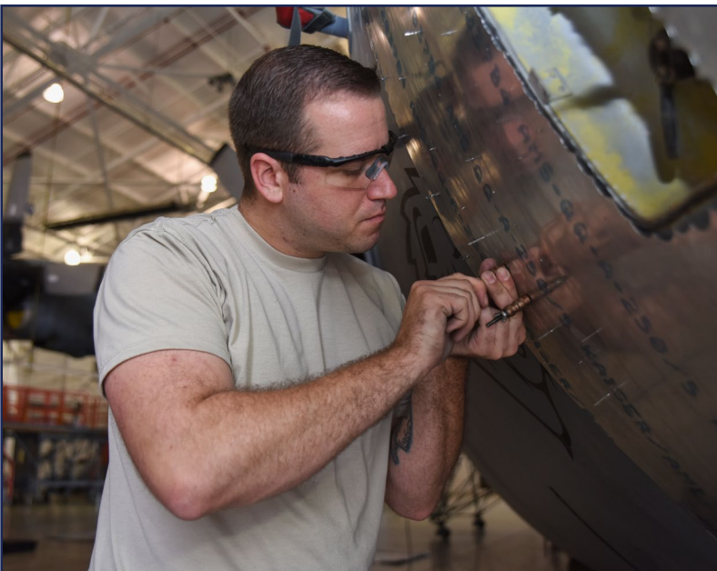
Staff Sgt. Robby Weng, aircraft structural repair mechanic, prepares a flush repair on a nose landing gear door. The repair was part of an extensive job replacing pieces of damaged skin of a C-130H.
