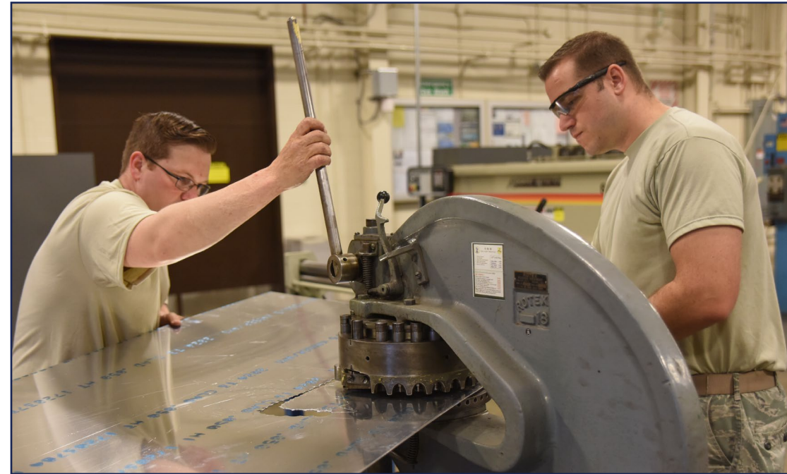
Tech. Sgt. Scotty Daniel and Staff Sgt. Joshua Chaplin cut a piece of sheet metal to be fitted and mounted onto a plane that sustained multiple areas of damage after a bird strike.
